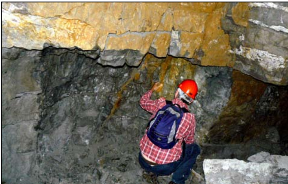
Undercutting of limestone beneath the chert bed in the Holme Bank mine, in the remains of a working face that was simply abandoned when the mine ceased operation.
